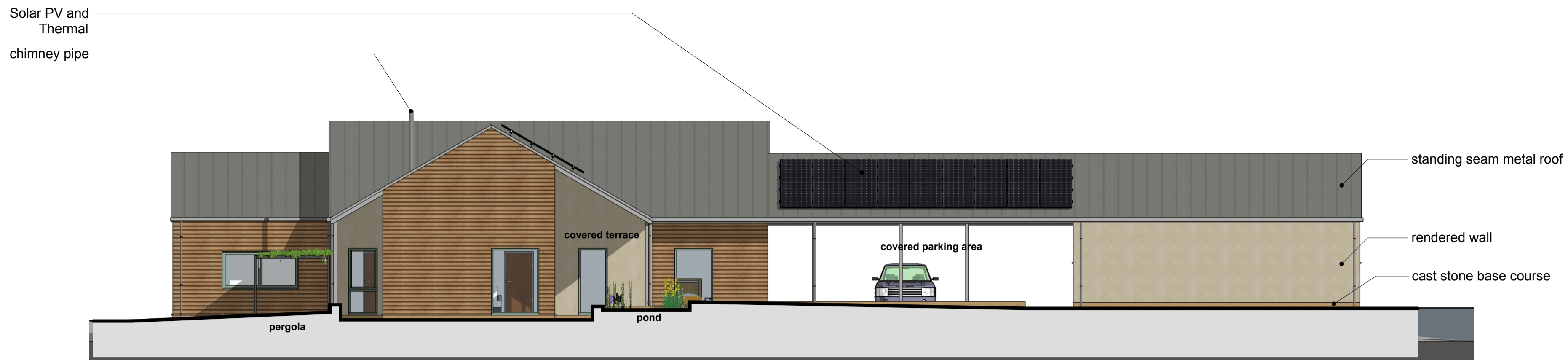
SOUTH WEST ELEVATION
